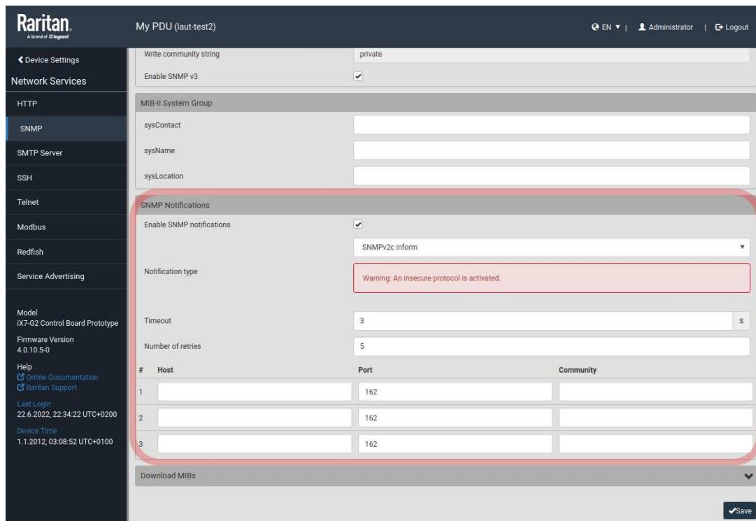
Figure 2: SNMP notification settings dialog of the web user interface
